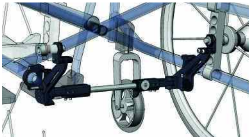
Example of mounting bracket for foldable wheelchair frame
