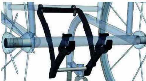
Example of mounting bracket for rigid wheelchair frame
